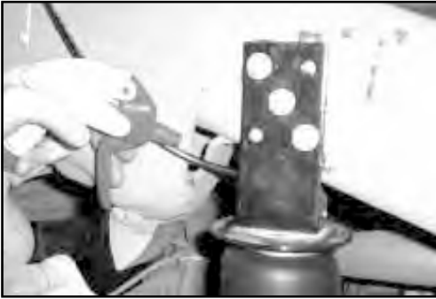
Leak test the air line connections and threaded connection of the elbow into the air spring. See page 11 to repair.
